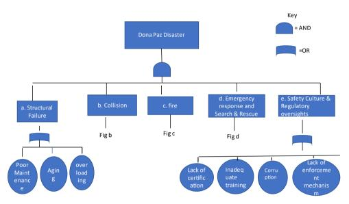
Figure 2. The Fault Tree Analysis of Doña Paz disaster
