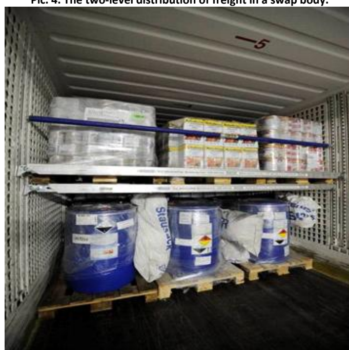
Pic. 4. The two-level distribution of freight in a swap body.
